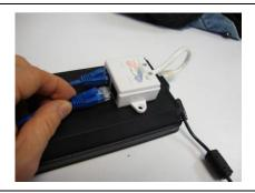
Sign output ports are labeled on the Control Box. Use one for each Scrolling Display.
