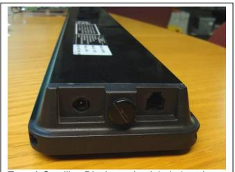
Type A Scrolling Displays: Are labeled on the back for use with "Use with 9 VAC". Type A signs also use a telephone cable (RJ11) for a data connection.
