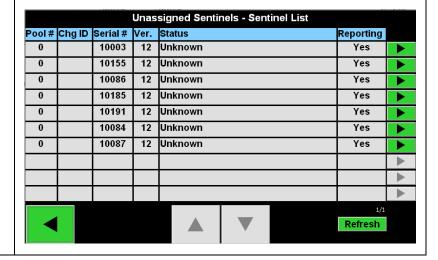
To find an unassigned Sentinel or determine if a Sentinel has been assigned properly, press Blue On. This will turn the blue LED on the Sentinel on. Press Blue Off when finished.
