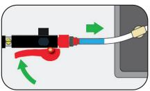
Squeeze the lever completely to fill the battery. **Do Not Partially Squeeze the Lever.**
