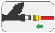
Attach the red hose to the white male end of the sediment filter. Do not use more than 20 ft. of hose
