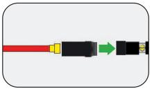
Attach the Instant Valve Pro™ to the end of the Pressure Regulator
