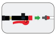
Release the lever and then disconnect the Instant Valve Pro from the Water Injector System.
