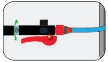
Watch the spinner mounted on the Instant Valve Pro. When it stops spinning, the filling is completed.
