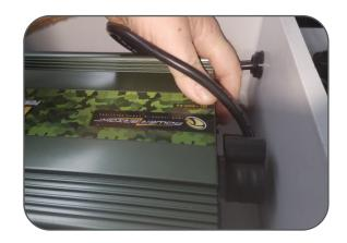
NOTE: Inverter will shut off when battery voltage reaches 20 VDC. If this occurs, fully charge the battery before the next use.
