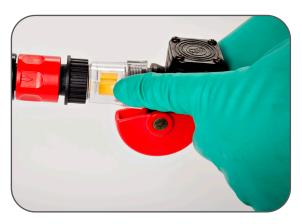
Watch the spinner mounted on the Instant Valve Pro. When it stops spinning, the filling is completed (about 15 seconds, usually). Note: The spinner may not come to a complete stop, especially in larger systems. The battery is filled when the spinner slows enough to clearly see the inner blades/ vanes.
