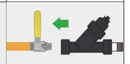
A Ball Valve with a 3/4" NPT male threaded fitting .must be plumbed in to a pressurized water line (>3/4" or more in diameter).
